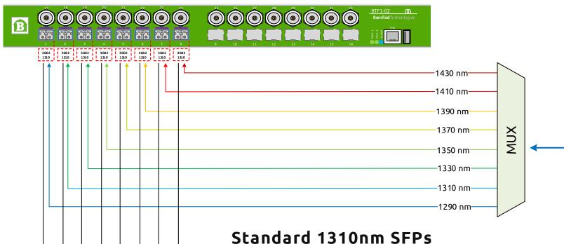
Frame equipped with standard 1310nm SFPs. The incoming optical signal has a different color on each channel. SFP receivers are universal for all colors. All signals with different colors are converted to 1310nm at the outputs of the BarnOne frame.
