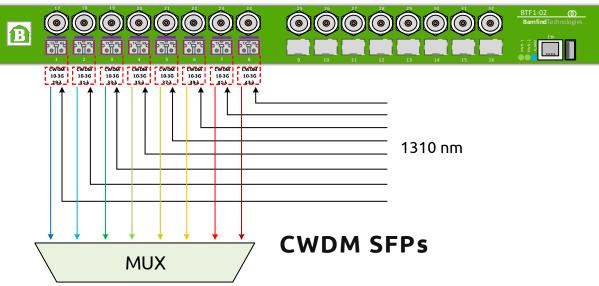
Frame equipped with CWDM SFPs. The incoming optical signal is 1310 nm on all channels. The signals are routed to an output with colored light. Each CWDM-SFP has a specific color on the transmitter.
